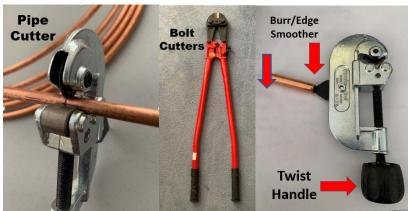
Measure 18" (45.72 cm) on the 36" inch long (91.44 cm) brazing rod and cut it. Take each rod and bend one end to make a ¾" (19.05 mm) "L". Use your pipe cutter to make a 4" (10.16 cm) length of copper tubing. You can also measure the palm of your hand to make it a comfortable, custom fit.
